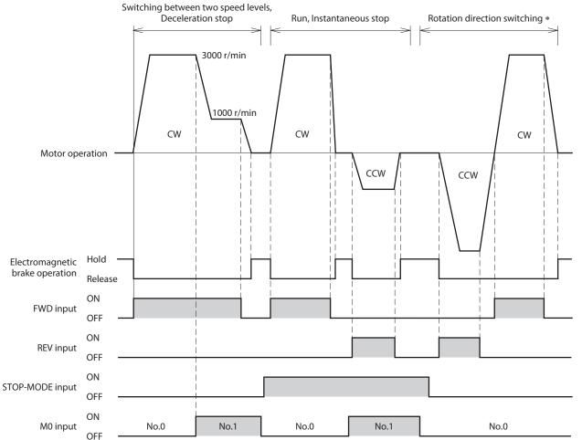
\* When the motor is combined with the **JH** gearhead, **JB** gearhead, or **JV** gearhead, the rotation direction cannot be switched instantaneously depending on the motor output. Check the operating manual of the motor.
