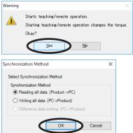
Note When the above window appears, all the communications in progress will be OFF. All the other monitors in progress in other windows are also stopped. Resume monitor after synchronization is completed.
