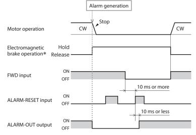
\* The electromagnetic brake will activate to hold the load at the moment an alarm generates. (The action of the electromagnetic brake can be changed with the "Electromagnetic brake function at alarm" parameter. However, do not change the parameter setting when using the motor in an application of vertical drive such as elevating equipment.)
