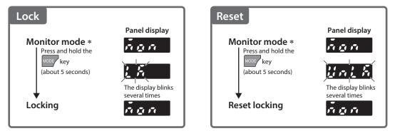
\* The edit lock function can be set when the top screen of each mode is displayed.
