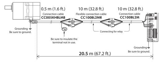
• Secure each connector part not to apply stress on the connector part. If not secured, the cables may damage due to stress.
