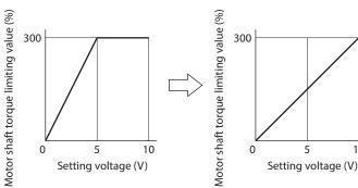
Analog torque limiting gain\* = Analog torque limiting Maximum value of setting voltage
