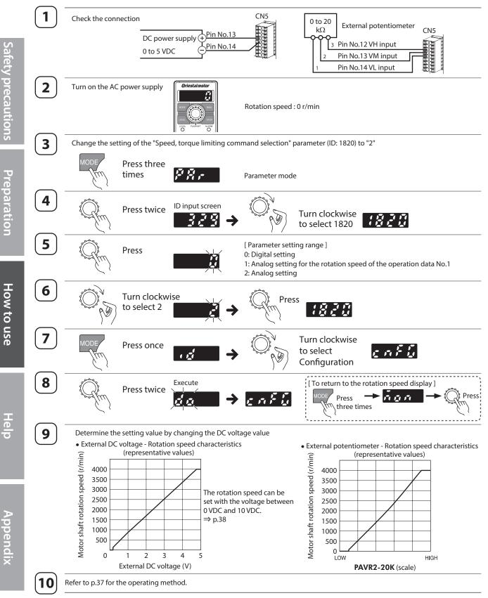
If the display is not shown as the above steps, check "Setting of parameters" of the operation panel on p.51.
