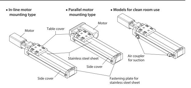
\* Only the in-line motor mounting type is available for the models for clean room use.
