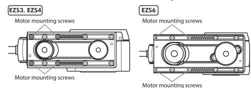
3. Change the cable leading direction, and mount the motor to tentatively fix the motor mounting screws. Tentatively fix the screws in a degree to be able to move the motor when touching it.
