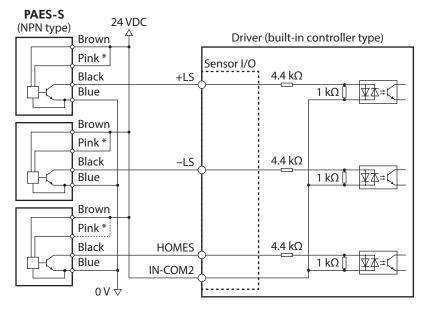
\* The logic of the sensor varies depending on the connection method. When the pink color lead is connected to the brown color lead, the sensor logic will be "normally closed."
