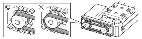
3. Attach the pulley cover, and tighten the screws. Tightening torque: 1.0 N·m (142 oz-in)
