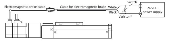
\* Be sure to connect the varistor to protect the contact of the switch or to prevent electrical noise. Motorized linear slide equipped with the **AZ** Series : Recommended varistor: Z15D121 (SEMITEC Corporation) Motorized linear slide equipped with the **AR** Series : Use the supplied varistor.
