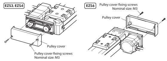
2. Check the the belt condition. And check the belt does not detach or protrude from the pulley.
