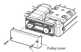
Pulley cover fixing screws Nominal size: M3
