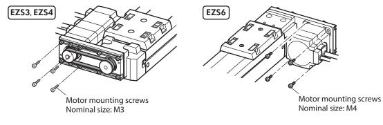
Do not loosen or remove the screws other than the motor mounting screws.
