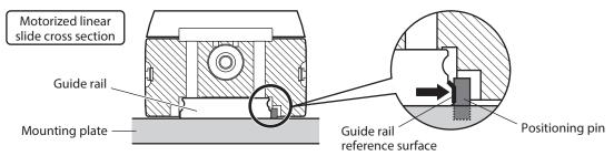
2. Use the mounting reference surface to position the X direction.
