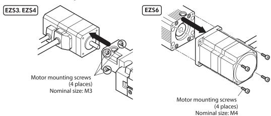
Change the cable leading direction, and mount the motor. Mount the motor according to the procedure opposite of dismounting it. Refer to the table below for the tightening torque of the coupling fixing screw and motor mounting screw.
