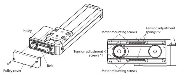
\*1 The motor is fixed in the position where the belt tension becomes optimum.
