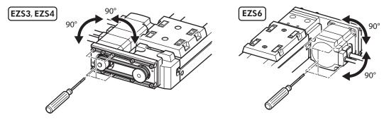
4. Loosen the tension adjustment screws. When loosening the screws, tension of the belt will be adjusted properly by the strength of springs.
