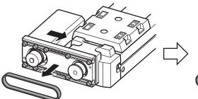
5. Tighten the motor mounting screws with pressing the motor in the direction of arrow so that the motor does not tilt.
