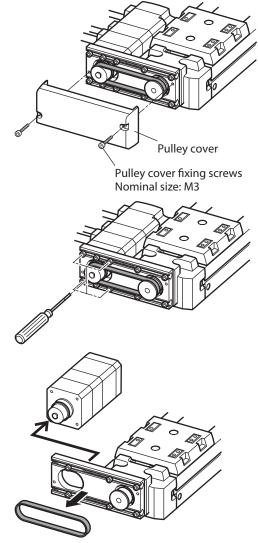
2. Remove the motor mounting screws.
