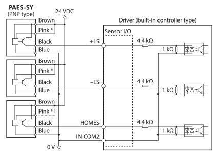
\* The logic of the sensor varies depending on the connection method. When the pink color lead is connected to the brown color lead, the sensor logic will be "normally closed."
