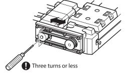
To prevent the tension adjustment screw from falling off, keep three turns or less when turning the screw.
